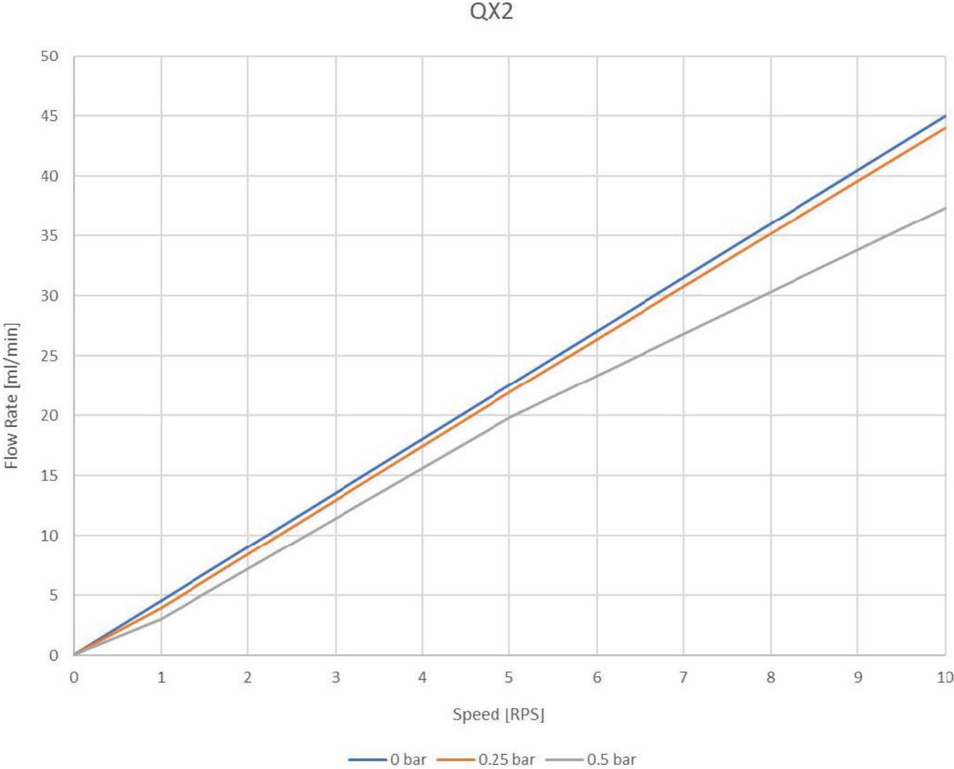
The 13mm rotor carries 3 cavities each with a volume of 0.21ml. Inlet and outlet ports are attached to an in-line system. The pump can be driven by a stepper or DC motor.
