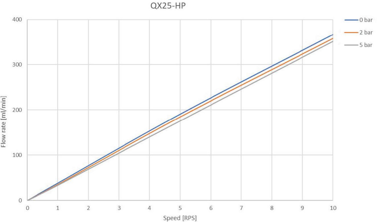
The 19mm rotor carries 3 cavities each with a volume of 0.50ml. This pump fits directly into a standard Bag-in-Box (BiB) gland and is compatible with most bag making and filling lines. The pump can be driven by a stepper or DC motor.
