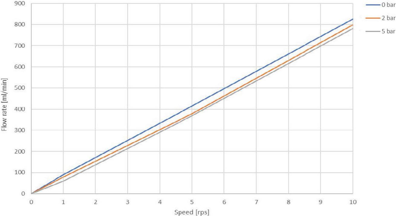
The 20mm rotor carries 2 cavities each with a volume of 1.35ml. . Suitable for high viscosity liquids and soft particulates. The pump can be driven by a stepper or DC motor.
