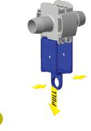
To complete the connection, simply snap the pull tabs together by pushing on the CPC logos and pull the membranes from the connector.
