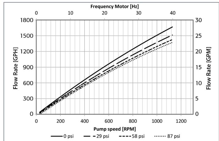
Depending on the selected motor/frequency drive combination, the motor frequency and the resulting pump speed might differ.
