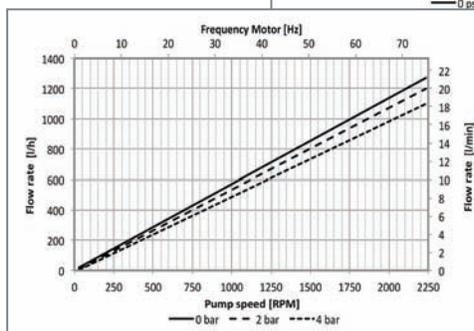
Depending on the selected motor/frequency drive combination, the motor frequency and the resulting pump speed might differ.
