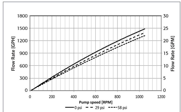
Depending on the selected motor/frequency drive combination, the motor frequency and the resulting pump speed might differ.
