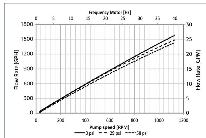
Depending on the selected motor/frequency drive combination, the motor frequency and the resulting pump speed might differ.
